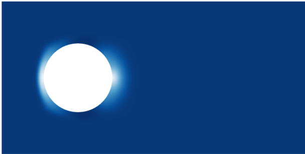
Figure 10: Velocity magnitude plot for the flow around the disk with a diameter of 0.9. Lighter colors indicate larger intensity.
