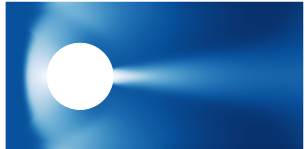
Figure 12: Velocity magnitude plot for the flow around the disk with a diameter of 0.9. Lighter colors indicate larger intensity.
