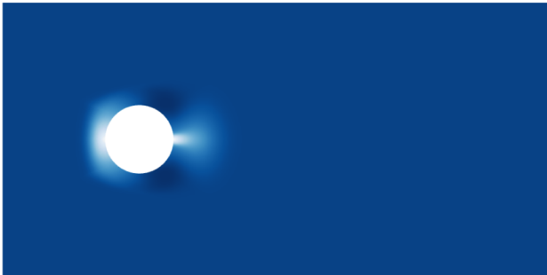
Figure 7: Velocity magnitude plot for the flow around the disk for mesh 2. Lighter colors indicate larger intensity.
